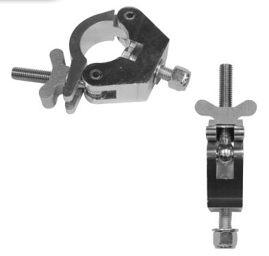
The CTC-50HCN is a load rated narrow half-coupler made from heavy duty aluminum with a load rating of 750 kg (1,650 lbs). Built with reliability, safety, and durability in mind, the CTC-50HCN is perfectly made for hanging fixtures and pipe structures from 2-inch pipes, including the CT290 series TRUSST® and other major brands in the market.
